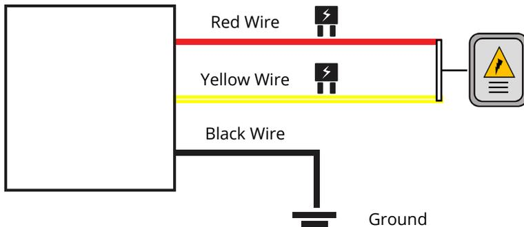
5. **Chassis ground-** Connect to TTU Black Wire, typically this is a white connection on the trailer harness.
