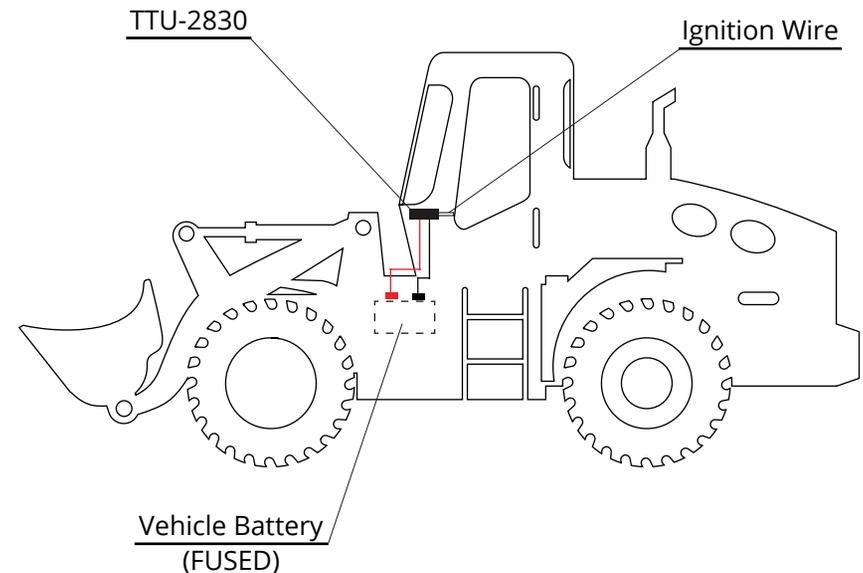
*\* Device and battery location may differ depending on vehicle model*
