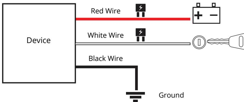
*Failure to connect these lines as described may result in discharge of the vehicle battery.*
