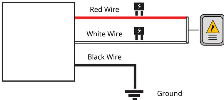
5. **Chassis ground-** Connect to TTU2830 Black Wire, typically this is a white connection on the trailer harness.
