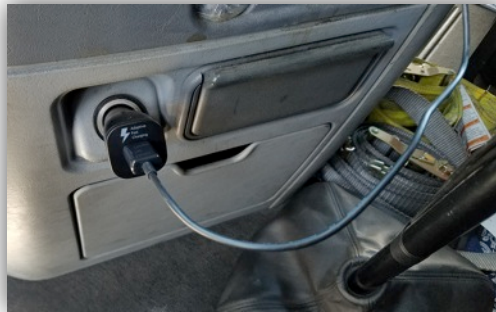
Plug tablet USB Cable into Cigarette Lighter
