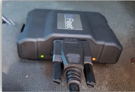
Connect Serial DB9 Pin End of the Vehicle Connector to the GPS Device
