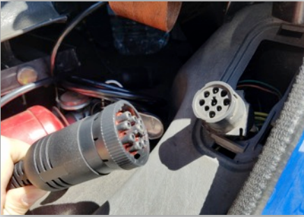
Connect Vehicle Connector Cable to the jBUS Connector
